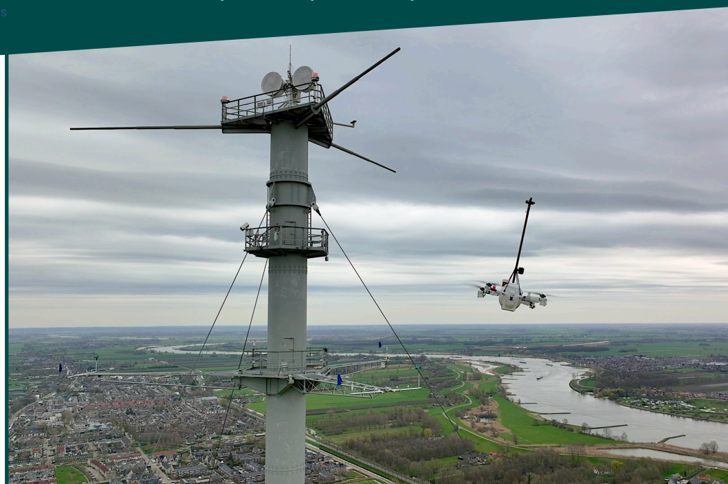
Figure 2: The MetSprite UAS hovering at the 200-m altitude of the KNMI Cabauw meteorological mast, tilting into wind.
