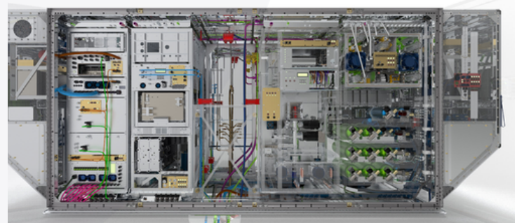
CAD drawing (partially transparent) of the new CARIBIC laboratory (width x height x depth = 406 x 162 x 153 cm, total weight: ~2.0 t), with the gas cylinder rack (right) and parts of the safety, communication and ventilation systems in the side compartments. The electrical and pneumatic connection to the A350 systems and the air inlet system occurs through the floor breakthrough in the middle section.
