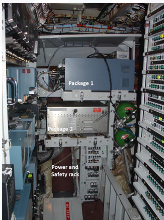
Fig. 1: IAGOS-CORE rack with instruments (P1, H 2 O, BCP and P2b) installed in an Airbus A340-300 operated by Lufthansa (left) and outside view of the IAGOS-CORE Inlet Plate (top).
