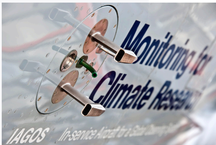
Fig. 1: IAGOS-CORE rack with instruments (P1, H 2 O, BCP and P2b) installed in an Airbus A340-300 operated by Lufthansa (left) and outside view of the IAGOS-CORE Inlet Plate (top).
