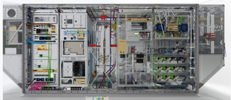
(above) CAD drawing (partially transparent) of the new CARIBIC laboratory (width x height x depth = 406 x 162 x 153 cm, total weight: ~2.0 t), with the gas cylinder rack (right) and parts of the safety, communication and ventilation systems in the side compartments. The electrical and pneumatic connection to the A350 systems and the air inlet system occurs through the floor breakthrough in the middle section.
