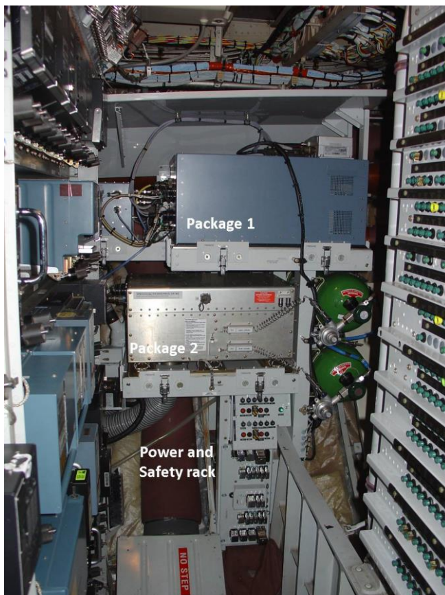
Fig. 1: IAGOS-CORE rack with instruments (P1, H 2 O, BCP and P2a) installed in an Airbus A340-300 operated by Lufthansa (left) and outside view of the IAGOS-CORE Inlet Plate (top).
