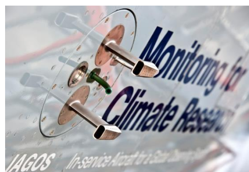
Fig. 1: IAGOS-CORE rack with instruments (P1, H 2 O, BCP and P2a) installed in an Airbus A340-300 operated by Lufthansa (left) and outside view of the IAGOS-CORE Inlet Plate (top).
