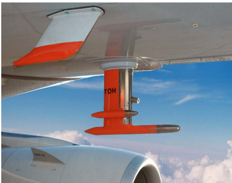
Fig. 2: Cargo container equipped with CARIBIC instruments (top) and the CARIBIC inlet mounted below the aircraft (left).
