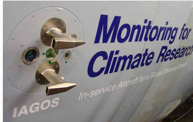
Figure 20: IAGOS inlet on the Lufthansa aircraft D-AIGT (Viersen).
