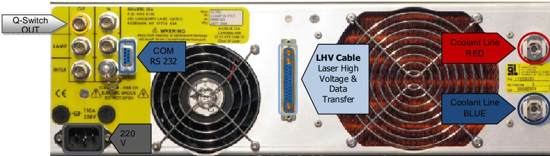
Figure 5: Back Panel of the Laser Unit (ICE)
