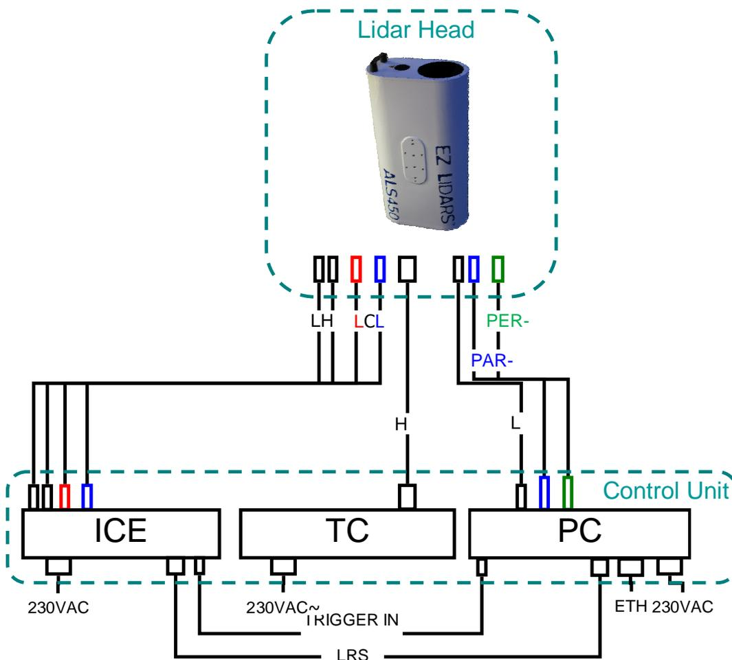
Figure 2: EZ LIDAR Block Diagram
