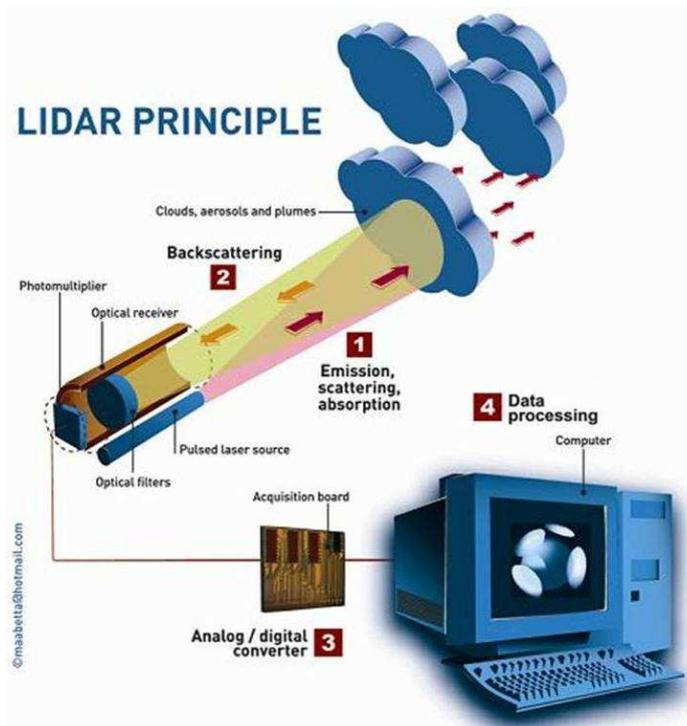
Figure 1: Measurement Principle of the EZ LIDAR
