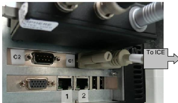
Figure 9: Back Panel of the Industrial Computer (All cables connected)
