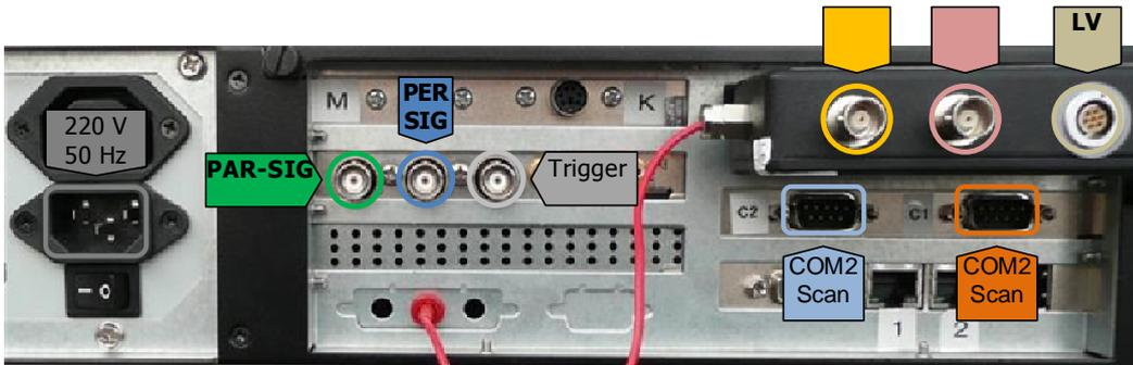
Figure 7: Back Panel of the Industrial Computer (no cable connected)
