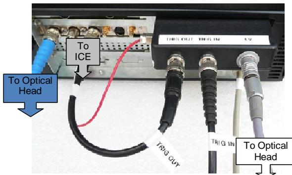
Figure 8: Back Panel of the Industrial Computer (All cables connected)
